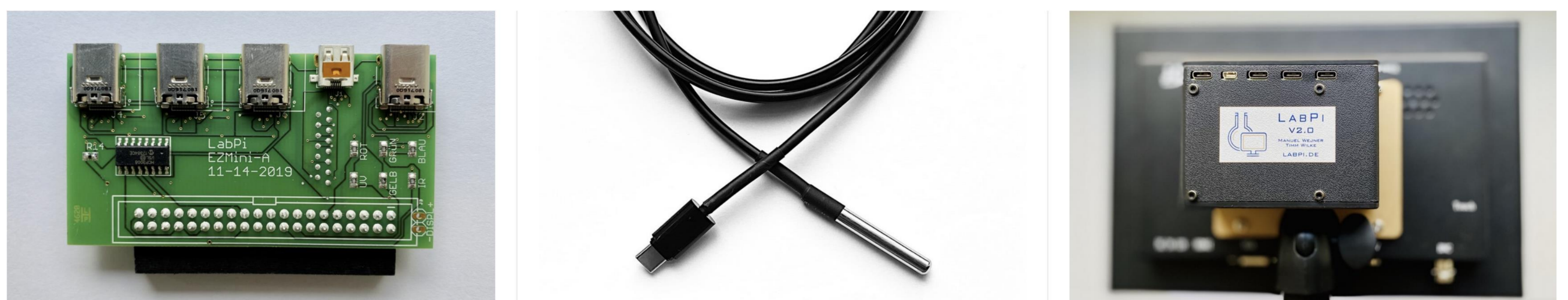
Fig. 2: Adapter Board (left), temperature sensor (middle) and the assembled LabPi-Station on a touch display (right).
